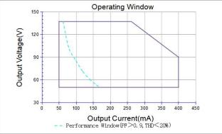
It's important to set the output current (AOC value) according to the LED voltage and make sure the power is within 36 W + 5%.
