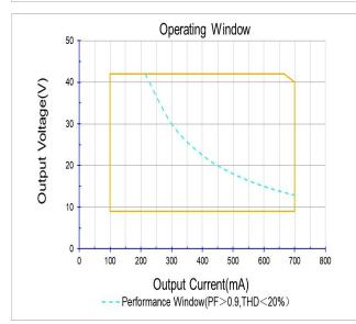
It's important to set the output current (AOC value) according to the LED voltage and make sure the power is within 28 W + 5%.
